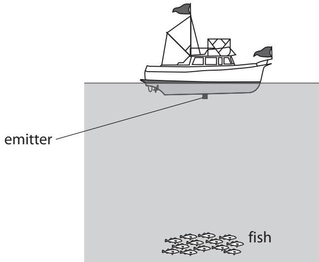
The high frequency sound waves travel from the emitter to the fish and then back to the emitter, where they are detected.
