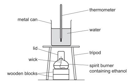
A student carries out an experiment to determine the value for  $\Delta H_c$  of ethanol using the following instructions:
